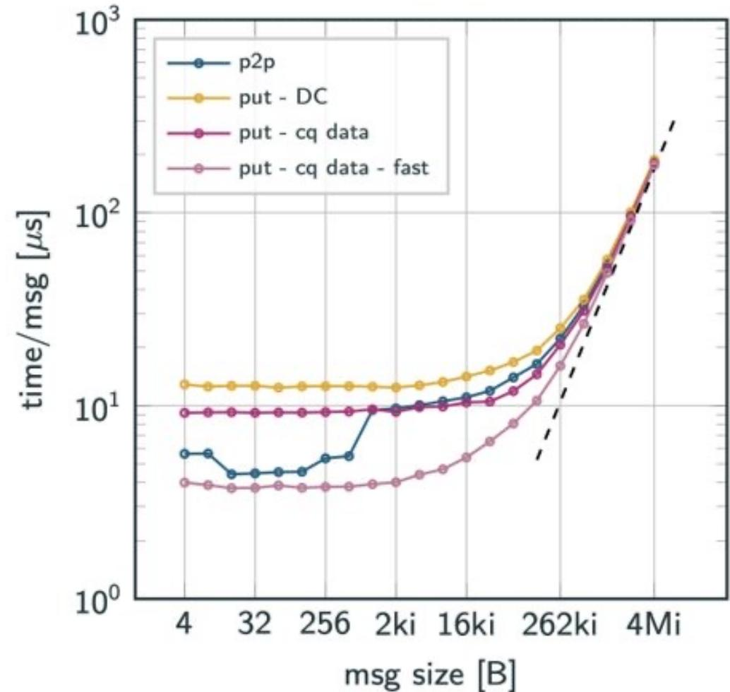
Latency for 1 msg (GPU-to-GPU)
